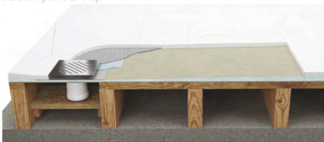
Square pre-formed tray and drain laid directly on floor boards
