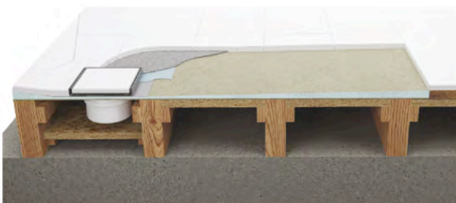
Square pre-formed tray and drain using underboarding, including under trap
